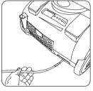
**NOTE:** Fully unwind the power cord. A yellow mark on the power cord indicates the recommended cord length. Do not exceed the cord length beyond the red mark.
